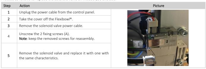
Proceed as follows to replace the solenoid valve on models 500, 650 and 800:
